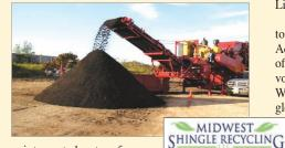
uninterrupted rate of more than 80 tons per hour. Shingles delivered to MSR's recycling facility are processed on-site while the portability of the grinder allows for offsite grinding of shingles that have been stockpiled, including "ground to order" production.
